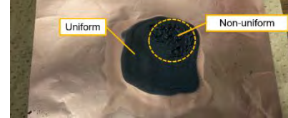
Fig. 5 Result of blasting process
