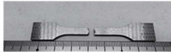
Fig. 12. Specimen TT-S150 after the tensile test.
